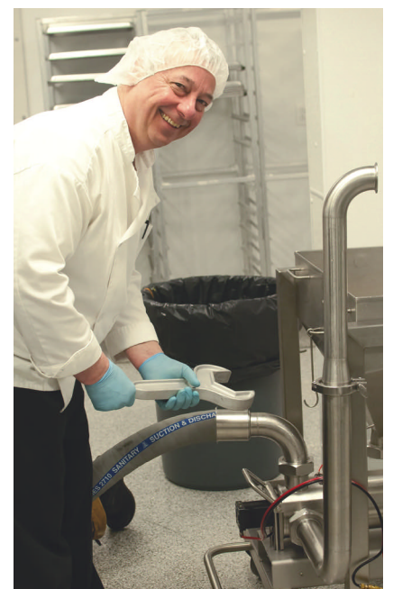
The soups are pumped from Hurricane's kettles to its filler. Above, Wilbur uses a wrench to connect the company's piston filler to one of its larger kettles.
