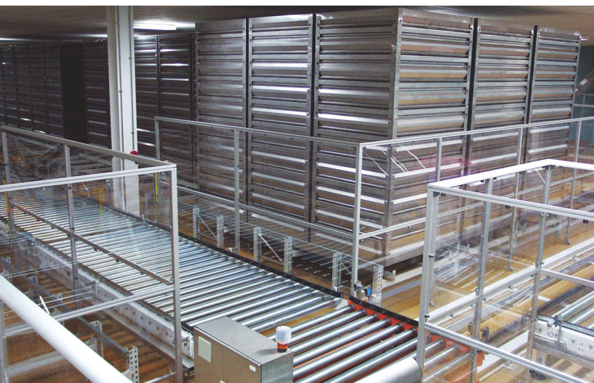
Filled trays are stacked vertically, and are then automatically placed into a storage system sized to meet the customer's inventory requirements.
